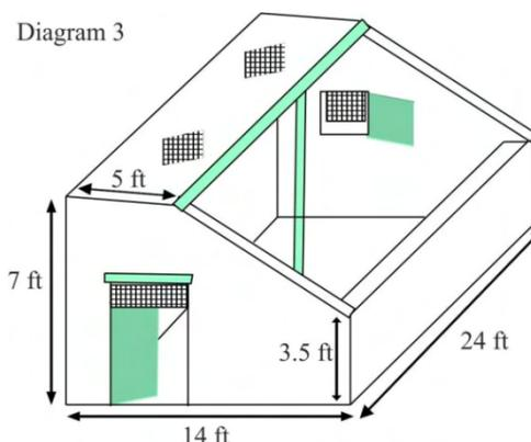
support the polythene sheet, joists are placed laterally every 5 ft, and wire is tied horizontally every 1.5 ft. This is necessary to support the polythene sheet and prevent it from being damaged by the wind. The polythene sheet should be fixed on a sunny day, so that it contracts as it gets cold and fits securely. The poly-sheet is secured with bags filled with mud both on the roof and on the side walls.
